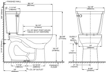
THIS TOILET IS DESIGNED TO ROUGH-IN AT A MINIMUM DIMENSION OF 254MM (10") FROM FINISHED WALL TO C/L OF OUTLET. SUPPLY NOT INCLUDED WITH FIXTURE AND MUST BE ORDERED SEPARATELY. \* DIMENSION SHOWN FOR LOCATION OF SUPPLY IS SUGGESTED.
